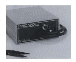
Set the energy level control to the desired value. LED and sonic indicators will alert operators when storage capacitor has charged to this level. Remember, when decreasing energy setting, that unit will retain last maximum energy level since discharge.
