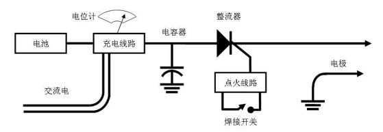
The system is powered directly from the AC line through a step-down transformer, or from a gel type storage battery. The storage battery is automatically recharged whenever the unit is connected to AC power. When the Hot Spot is turned on, the capacitor charging circuit charges the large energy storage capacitor to the level set by the level control.
