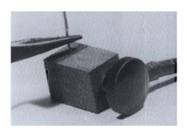
• Stripped wire pairs should be positioned in the plier electrode so that each wire is contacted. Asymmetrical contact can produce a distorted bead. Other factors, including wire material, contribute to bead distortions. Multiple attempts with the same junction may help in producing the desired shape.
