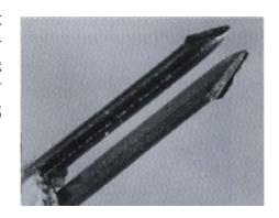
Heavy wires can be welded singly to metal base parts. Lighter wires can be welded in pairs. Using a carbon block allows free-standing bead type junctions to be formed Squeeze pliers firmly.
